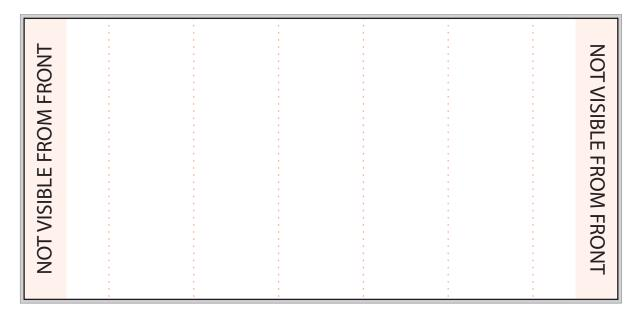
Pop Up displays stands will need an external bleed of 20mm at full size. On the diagram above this is shown as the grey area. The black line is the artwork size at 4711mm x 2230mm. The dotted lines indicate the panel splits of 673mm.
