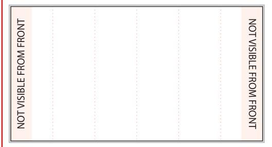
Pop Up display stands will need an external bleed of 20mm at full size. On the diagram to the left this is shown as the grey area. The black line is the artwork size at 4038mm x 2230mm. The dotted lines indicate the panel splits of 673mm.
