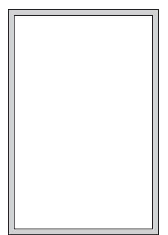
A double crown sized poster should have a safe area of 40mm internal bleed where there is no text or important images. This is shown on the diagram in grey. The safe area measures 468mm x 722mm.
