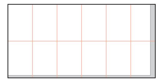
48 sheets require 4 inches on the bottom and 8 inches on the far right hand side which contains no text or important images, this is indicated on the diagram in grey. Once you have supplied us the artwork it will be printed with panel splits measuring 1016mm x 1524mm at full size making 12 panels in total. We take care of this.
